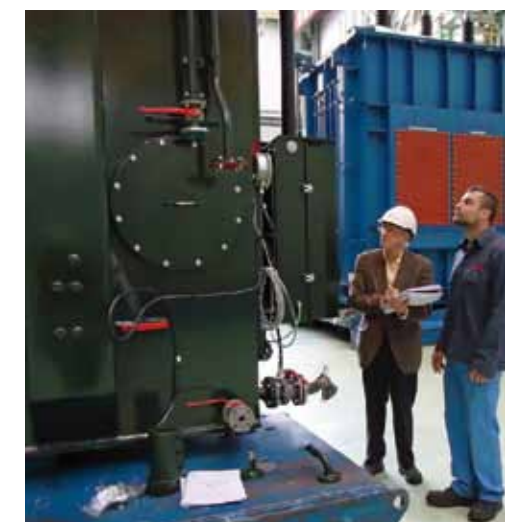
220/2 x 27.5 kV, 30 MVA power transformers.
