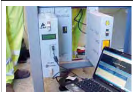
DOWNLOADING LOGS. Data can be downloaded from the logger, either 'in situ' or remotely, from a terminal station.
