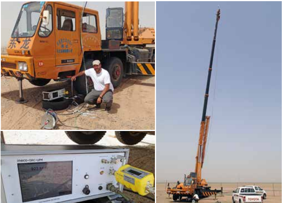
In the top left image, Ineco engineer, Alberto Trujillo, with a signal strength meter; bottom left, the radio transmitter designed by the SPRING team. To the right, an antenna on a crane.
