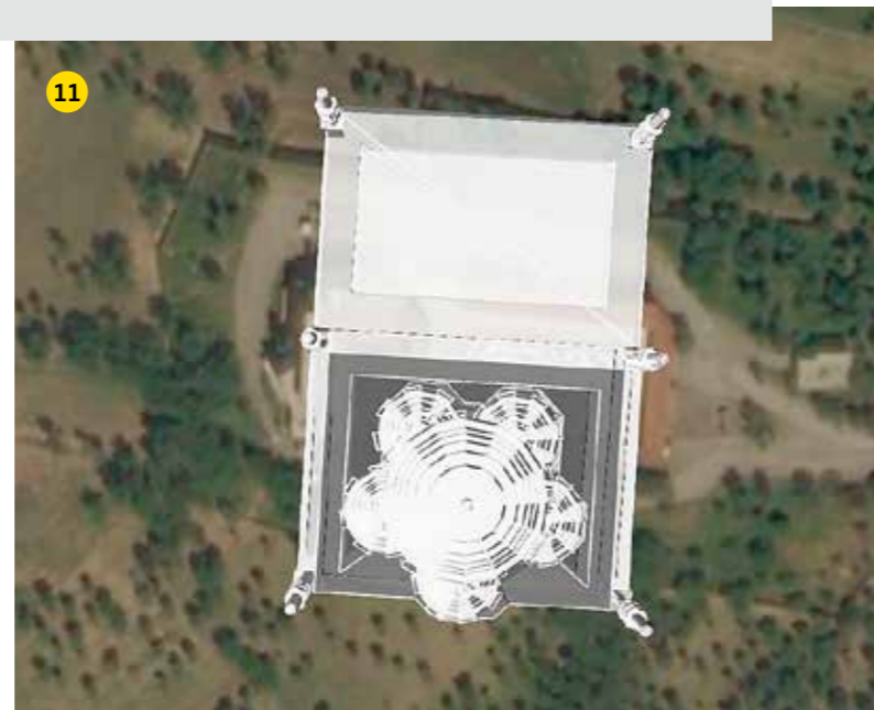
Figure 10 / Figure 11 / Figure 12. Elevation and plan views of the 3D model of the mosque used for the TACAN simulations carried out with Navtools.
