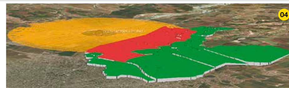
Figure 1. Location of the planned residential development under study with respect to Batman Airport and its CNS facilities (Google Earth). Figure 2. Model of the planned urban development created using Navtools for the simulation of pulsed systems. Figure 3. On-site representation and analysis of the BRA of Batman Airport's CVOR BAT equipment. Figure 4. 3D representation and analysis of the BRA of Batman Airport's CVOR BAT equipment. Image created with Navtools.
