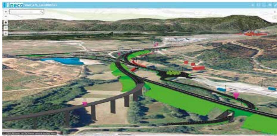
BIM-GIS DISPLAY ON A HIGHWAY. Image of the BIM-GIS integration display, which offers an overview of the 'digital twin' of the slip road between the future A-76 motorway and the A-6.
