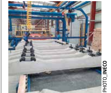
Plant to manufacture sleepers for the works.
